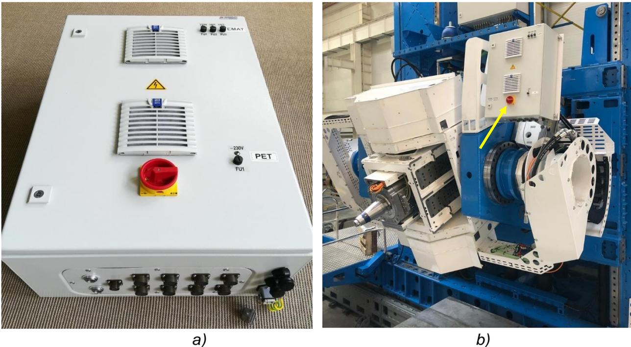
*Fig. 3 – Test Electronics Unit. a) Overall view b) SONAFLEX-FSW as a part of friction stir welding machine*
