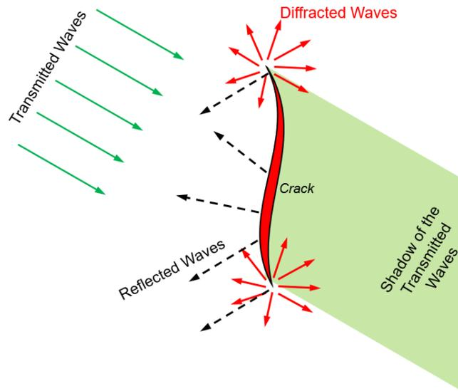
Fig. 6 – Physical basic of Diffraction Methods. Interaction of transmitted waves with crack
