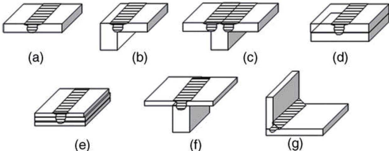
*Fig. 2 – Joint configurations for friction stir welding: (a) square butt, (b) edge butt, (c) T butt joint, (d) lap joint, (e) multiple lap joints, (f) T lap joint, and (g) fillet joint*
