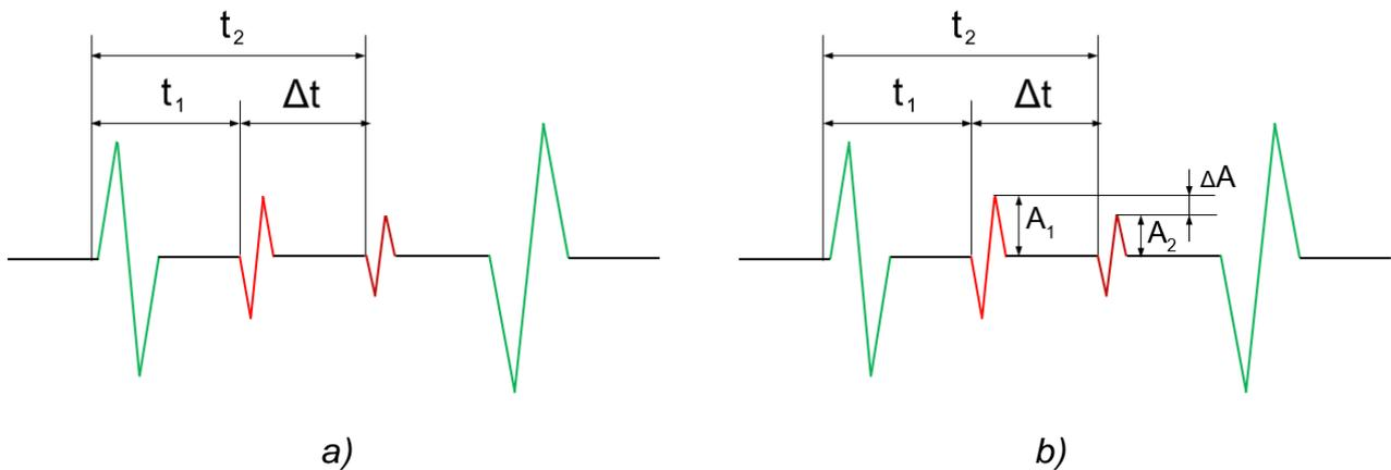
Fig. 8 – Informative parameters of the received signals for the Time-of-Flight diffraction Method (a) and Amplitude-and- Time-of-Flight diffraction Method (b)
