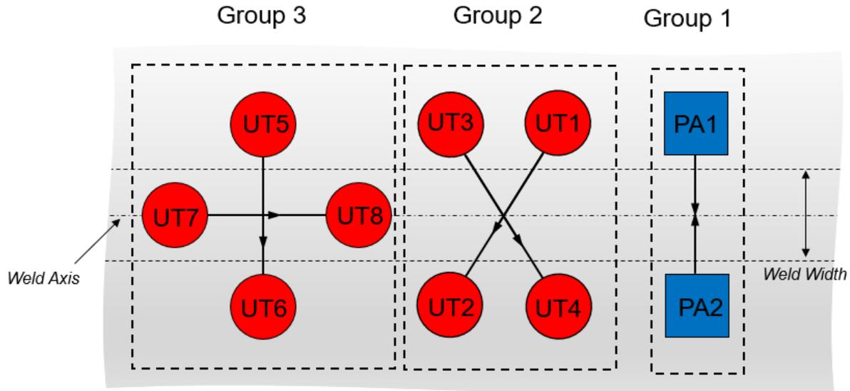
Fig. 4 – General Layout of the SONAFLEX-FSW probes. In Figure: Group 1 represented by two Phased Array Probes – PA 1 and PA 2, Groups 2 and 3 represented by eight angle beam assembling for performing TOFD/ATOFD configuration.
