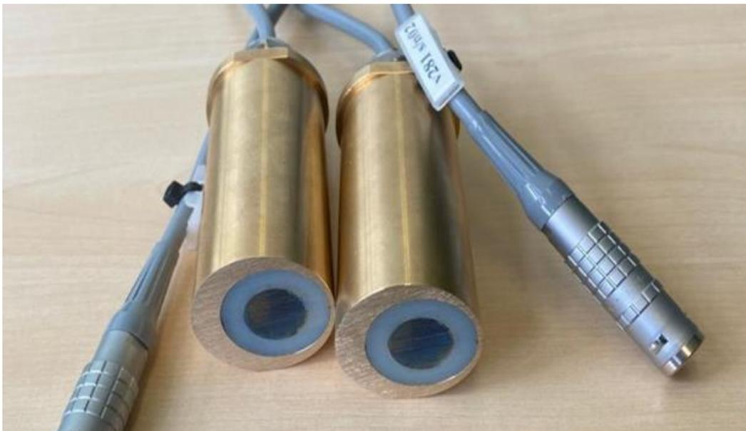
Fig. 9 – Overall View of Angle Beam Probes (remark: PA probes has similar overall view)
