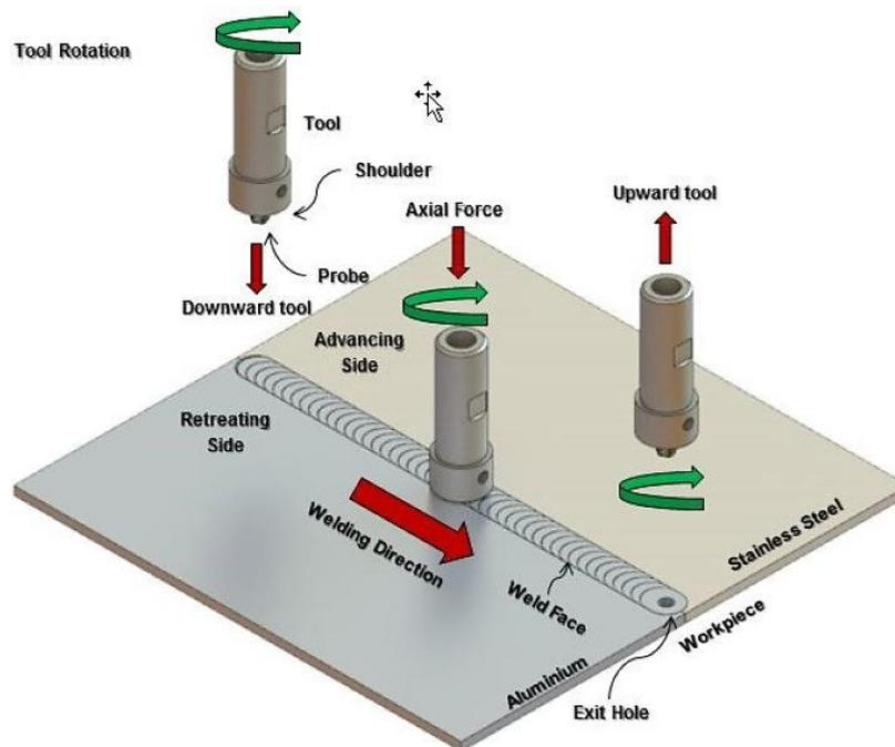
*Fig. 1 – Friction Stir Welding Procedure*
