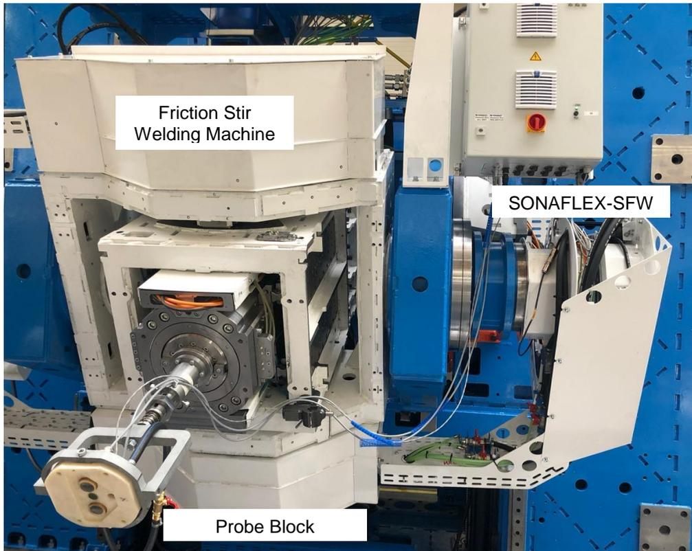
*Fig. 14 – Example of SONAFLEX-SFW integrated with Friction Stir Welding Machine. In this example, the UT probe block is fastened directly to the Welding head*
