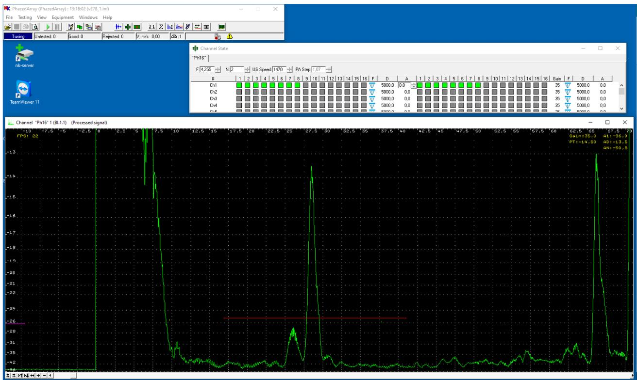
*Fig. 10 – Example of SONAFLEX-FSW main Window, Channels Control Window and A-scan obtained for surface notch 0.2 mm deep*
