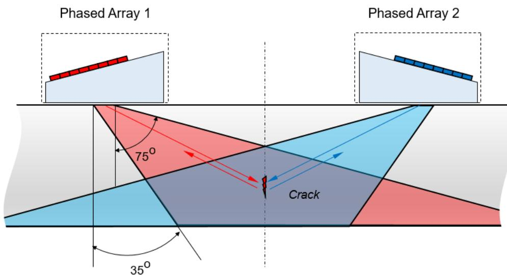
Fig. 5 – Applied Configuration Phased Array Probes and principles of defects detection
