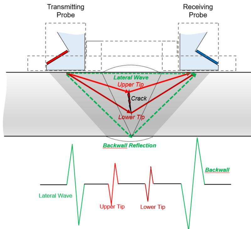
Fig.7 – Applied Configuration of Angle beam probes for realization of TOFD / ATOFD methods
