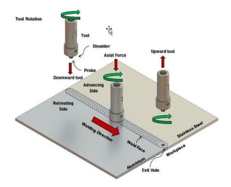
Fig. 1 – Friction Stir Welding Procedure
