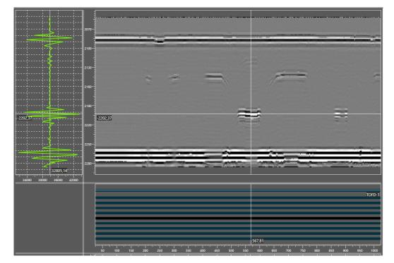
Fig. 12 – Example of SONAFLEX-FSW Presentation of A-Scan for TOFD system. Presentation of A, B and C-scans
