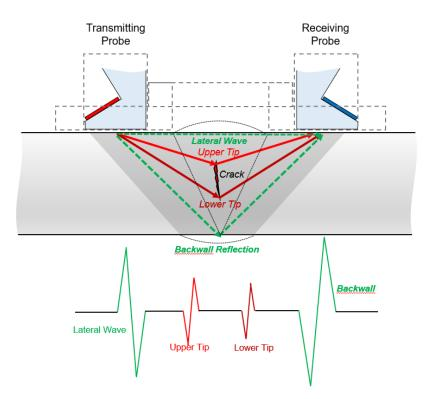
Fig.7 – Applied Configuration of Angle beam probes for realization of TOFD / ATOFD methods
