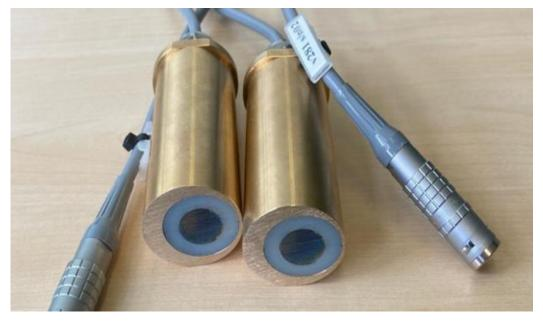
Fig. 9 – Overall View of Angle Beam Probes (remark: PA probes has similar overall view)
