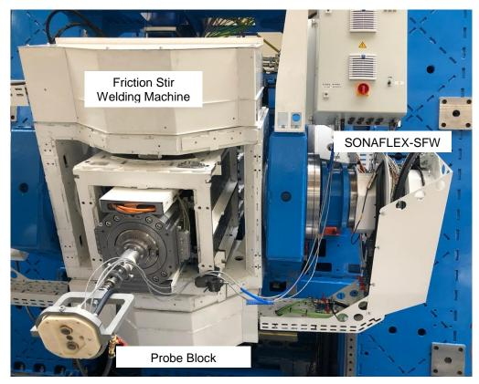
Fig. 14 – Example of SONAFLEX-SFW integrated with Friction Stir Welding Machine. In this example, the UT probe block is fastened directly to the Welding head
