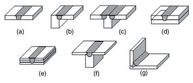
Fig. 2 – Joint configurations for friction stir welding: (a) square butt, (b) edge butt, (c) T butt joint, (d) lap joint, (e) multiple lap joints, (f) T lap joint, and (g) fillet joint
