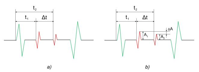
Fig. 8 – Informative parameters of the received signals for the Time-of-Flight diffraction Method (a) and Amplitude-and- Time-of-Flight diffraction Method (b)
