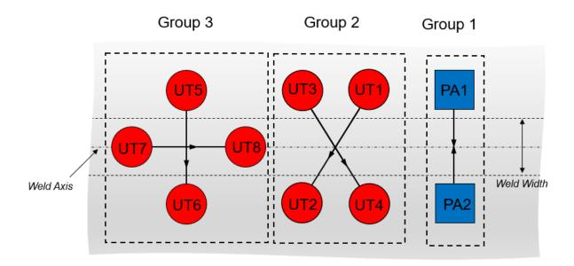
Fig. 4 – General Layout of the SONAFLEX-FSW probes. In Figure: Group 1 represented by two Phased Array Probes – PA 1 and PA 2, Groups 2 and 3 represented by eight angle beam assembling for performing TOFD/ATOFD configuration.
