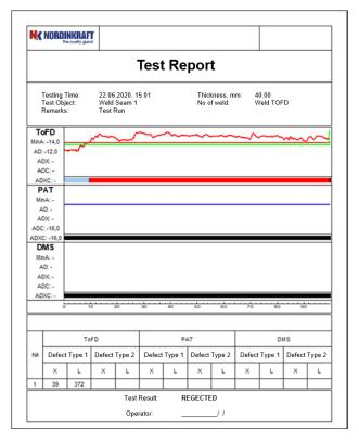
Fig. 13 – Example of the Test Report
