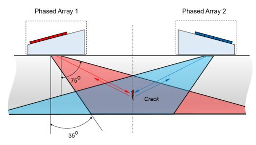
Fig. 5 – Applied Configuration Phased Array Probes and principles of defects detection
