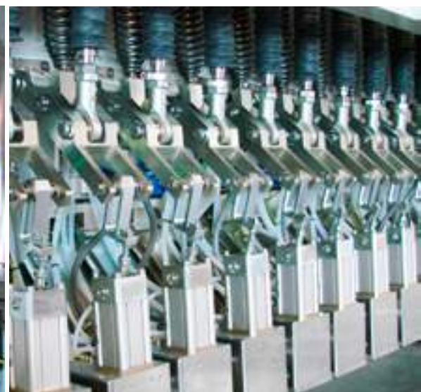
Blocks of EMATs made by Nordinkraft NDT Group for ultrasonic plate inspection. They can resist temperatures of up to +650 °C.
