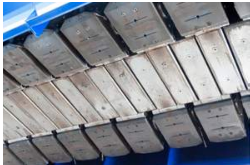
Blocks of EMATs assembled with magnetic systems.
