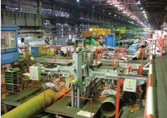
Fig.16. EMATEST-PIPE for longitudinal pipes inspection. Two systems for acceptance testing EMATEST-PIPE are located in parallel with each other in the production line «820» - Chelyabinsk Tube Rolling Plant, Chelyabinsk (Russia).
