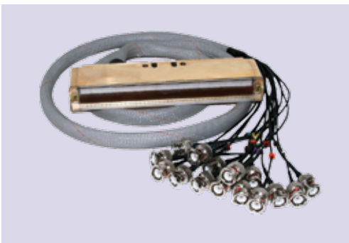
Fig.1. Piezoelectric probe for weld inspection.
