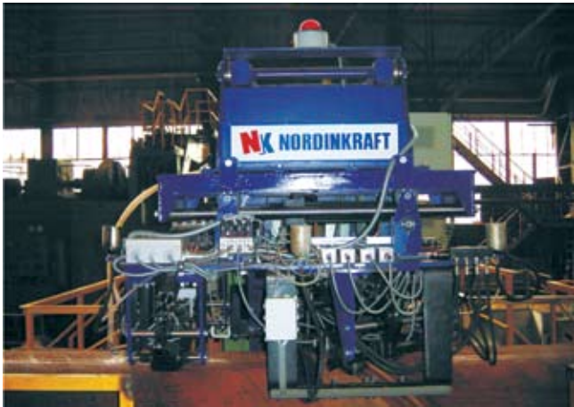
Fig.18. Measuring unit with electromagnetic acoustic transducers (noncontact).
