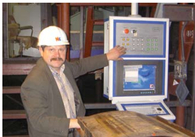
6 Fig.13. Control desk of the system EMATEST-PIPE - Chelyabinsk Tube Rolling Plant, Chelyabinsk (Russia).
