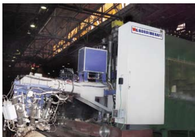
Fig.11. EMATEST-PIPE for ultrasonic inspection of spiral welded pipes - Volzhsky Pipe Plant, Volzhsky (Russia).
