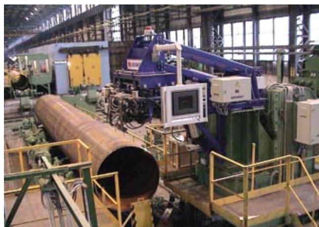
Fig.14. EMATEST-PIPE for ultrasonic inspection of spiral welded pipes - Volzhsky Pipe Plant, Volzhsky (Russia).
