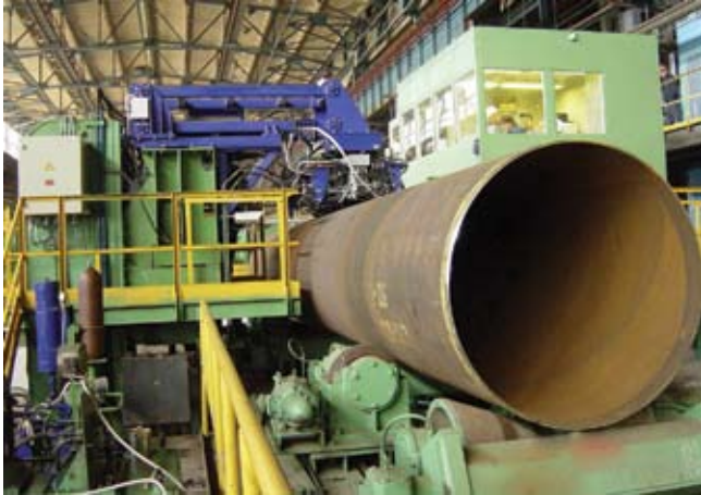
Fig.15. EMATEST-PIPE for ultrasonic inspection of spiral welded pipes - Volzhsky Pipe Plant, Volzhsky (Russia).
