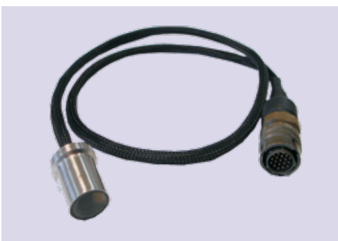
Fig.3. Piezoelectric phased array for weld inspection.
