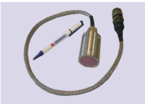
Fig.2. Electromagnetic acoustic transducer for weld (1,0 MHz) and ends inspection (5,0 MHz).
