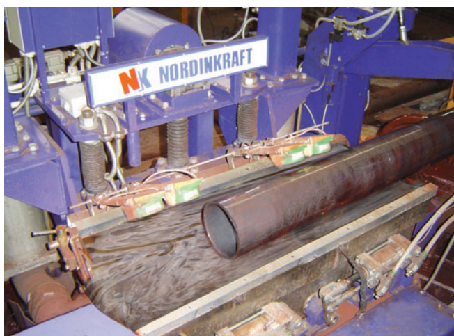
Fig.13, 14. «EMATEST-TU-8» for ultrasonic inspection of seamless tubes. Synarsky Pipe Works, Kamensk-Uralsky (Russia).
