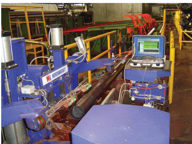
Fig.13, 14. «EMATEST-TU-8» for ultrasonic inspection of seamless tubes. Synarsky Pipe Works, Kamensk-Uralsky (Russia).
