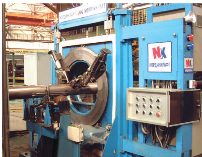
Fig.1. «EMATEST-TU-7» for ultrasonic testing of longitudinal welded tubes. Uraltrubprom, Pervouralsk (Russia).
