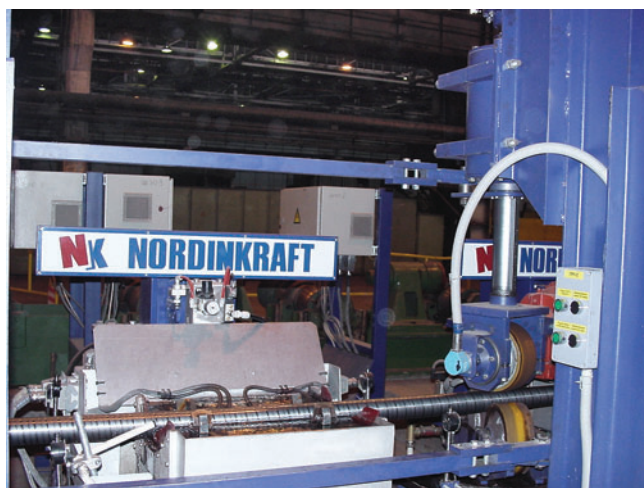
Fig.16. «EMATEST-TU-8» for ultrasonic inspection of seamless tubes. Volzhsky Pipe Plant, Volzhsky (Russia).
