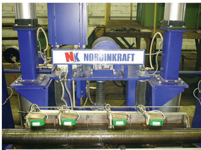
Fig.15. «EMATEST-TU-8» for ultrasonic inspection of seamless tubes. Volzhsky Pipe Plant, Volzhsky (Russia).
