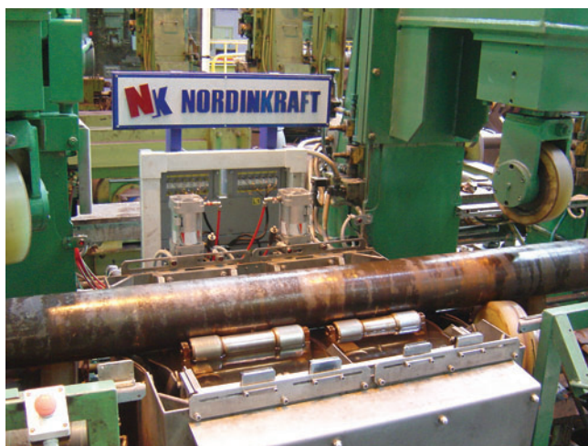
Fig.12. UTE «EMATEST-TU-8» for ultrasonic inspection of seamless tubes. Volzhsky Pipe Plant, Volzhsky (Russia).
